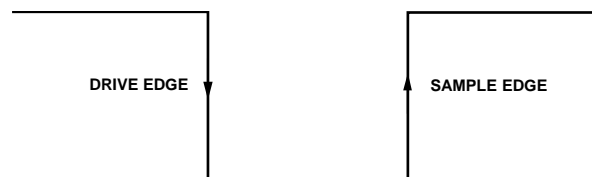
Figure 65. SPI Mode 3, SCLK Edges
