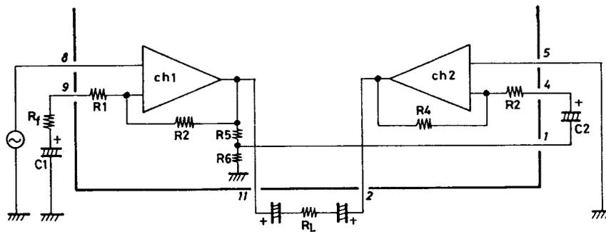
The above shows the bridge amplifier configuration, where ch.1 operates as a noninverting amplifier and ch.2 as an inverting amplifier. The output of ch.1 is divided with R5, R6 and led to pin 1 and then input to ch.2.
