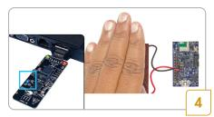
• Cover the Solar Module for five seconds with your hand, and notice the blue LED on the BLE-USB Bridge will no longer blink. When you remove your hand from the Solar Module, the blue LED will blink again
