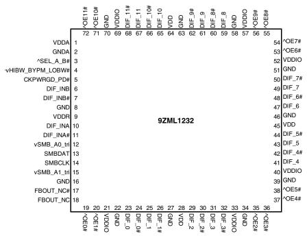
^ prefix indicates internal 120Kohm Pull Up v prefix indicates internal 120Kohm Pull down 10mm x 10mm 72-MLF, 0.5mm pin pitch
