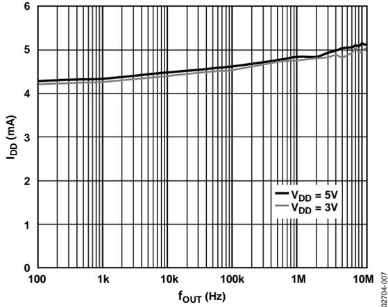
Figure 7. Typical  $I_{DD}$  vs.  $f_{OUT}$  for  $f_{MCLK} = 25$  MHz
