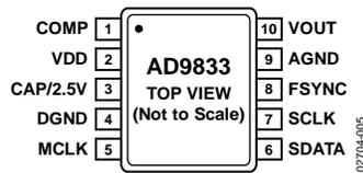
Figure 5. Pin Configuration
