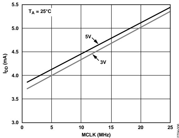
Figure 6. Typical Current Consumption vs. MCLK Frequency for  $f_{\text{OUT}}$  of MCLK/10
