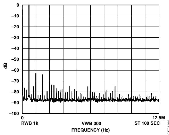
Figure 19.  $f_{MCLK} = 25 \text{ MHz}$ ,  $f_{OUT} = 600 \text{ kHz}$ , Frequency Word = 0x0624DD3
