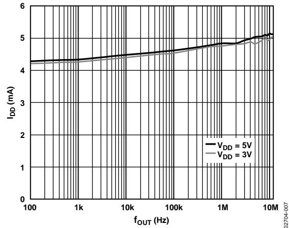
Figure 7. Typical  $I_{DD}$  vs.  $f_{\text{OUT}}$  for  $f_{\text{MCLK}} = 25\text{ MHz}$
