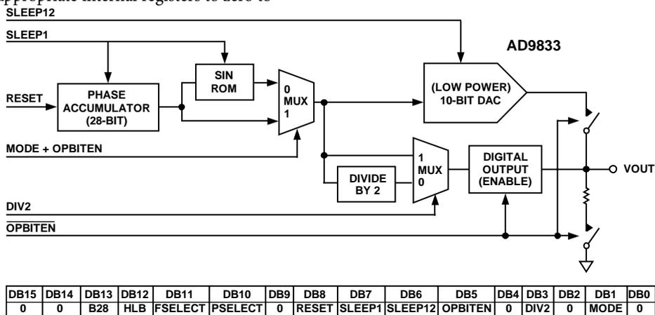
Figure 24. Function of Control Bits
