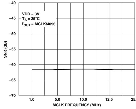
Figure 11. SNR vs. MCLK Frequency
