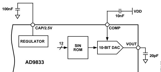
Figure 2. Test Circuit Used to Test Specifications
