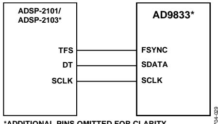
Figure 29. ADSP-2101/ADSP-2103 to AD9833 Interface
