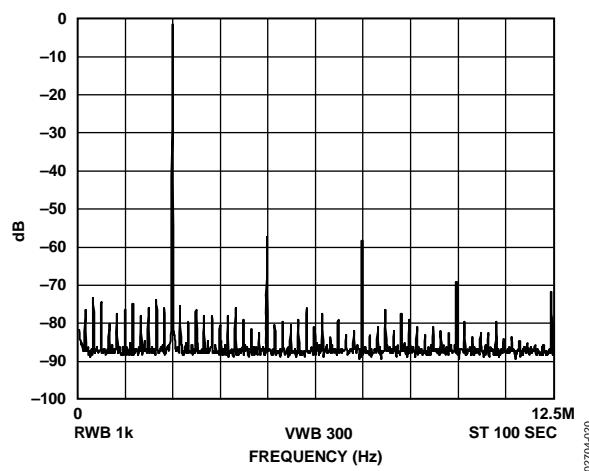
Figure 20.  $f_{MCLK} = 25 \text{ MHz}$ ,  $f_{OUT} = 2.4 \text{ MHz}$ , Frequency Word = 0x189374D
