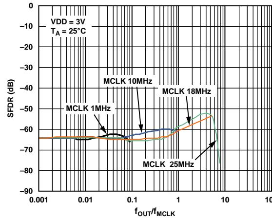
Figure 10. Wideband SFDR vs.  $f_{\text{OUT}}/f_{\text{MCLK}}$  for Various MCLK Frequencies
