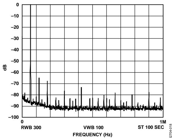
Figure 18.  $f_{MCLK} = 25 \text{ MHz}$ ,  $f_{OUT} = 60 \text{ kHz}$ , Frequency Word = 0x009D495
