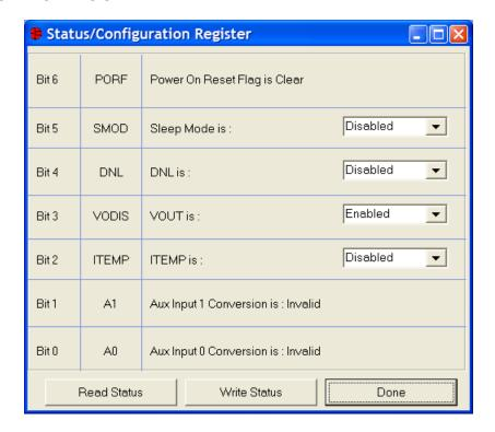
The present state of all register bits are displayed immediately upon opening the register window. R/W locations contain a selection field or command button to allow the user to determine their state. Pressing the Write Status button will write the new value to the register and read the corresponding register inside the DS2786 to verify the correct value was written. Note: This window does not copy these values to EEPROM. To copy the desired values to EEPROM, see the Parameters section.
