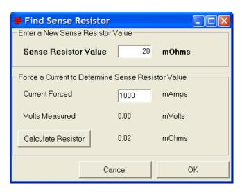
The sense resistor value used to calculate the current reading is shown in the current section. Left-click on the Update Sense Resistor button to open the Find Sense Resistor window.
