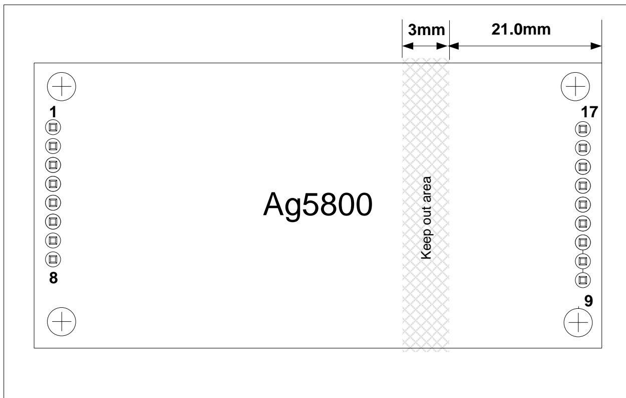
Figure 17: Position of the Isolation Barrier
