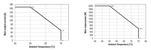
Figure 21. Maximum current and power levels PET2000-12-074ND
