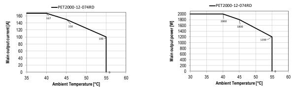
Figure 22. Maximum current and power levels PET2000-12-074RD
