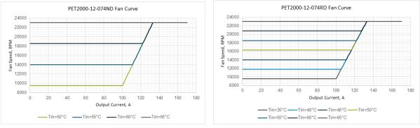
Figure 20. Fan speed vs. main output load
