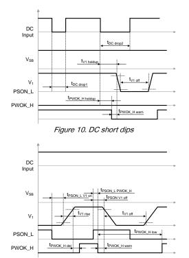
Figure 12. PSON\_L turn-on/off timing
