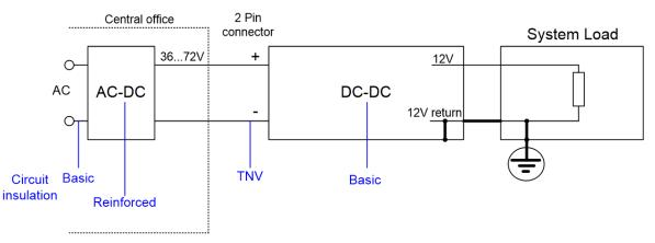
Figure 5. Block diagram with reliable System Earth connection
