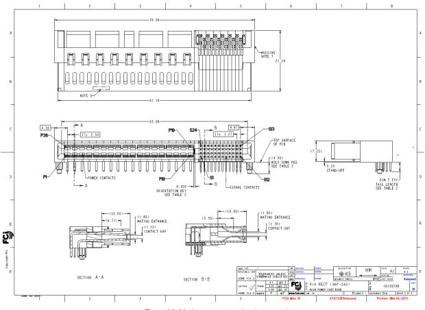
Figure 28. Mating connector drawing page 1
