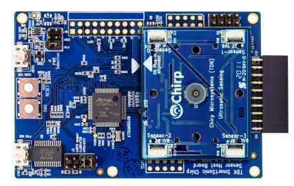
Part of the SmartSonic platform, the DK-CH201 is designed around Atmel's SAMG55 Cortex-M4 MCU, and can be used by developers for rapid evaluation and development of CH201 based solutions. The DK-CH201 includes an on-board Embedded Debugger so external tools are not required to program or debug the SAMG55 MCU. The DK-CH201 includes an on-board Embedded Debugger so external tools are not required to program or debug the SAMG55 MCU.
