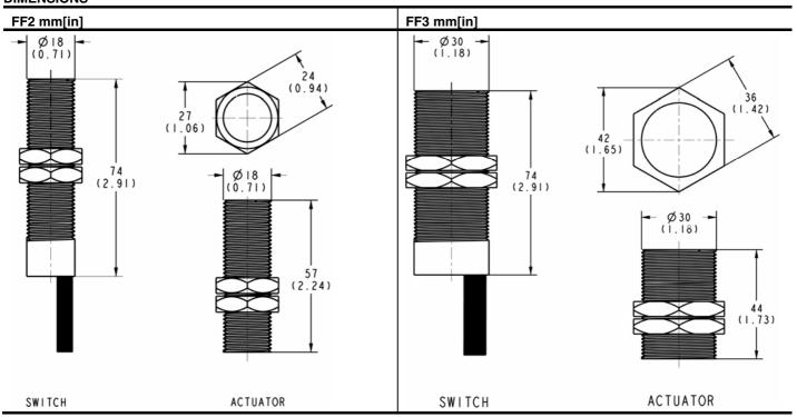
Magnetically Actuated Non-Contact Barrel Safety Switches
