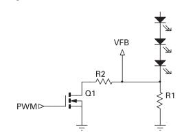
$$MOSFET 'off' \\ I_{LED(MIN)} = \frac{V_{FB}}{R_{LED}}$$
