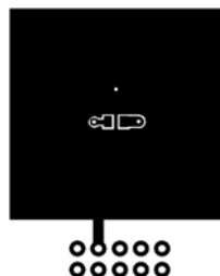
a) 80\text{ }^\circ\text{C/W} when mounted on a 1\text{ in}^2 pad of 2 oz copper
