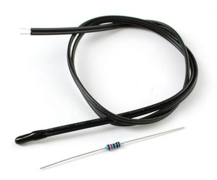
There are two kinds of of thermistors, NTC (negative temperature coefficient) and PTC (positive temperature coefficient). In general, you will see NTC sensors used for temperature measurement. PTC's are often used as resettable fuses - an increase in temperature increases the resistance which means that as more current passes through them, they heat up and 'choke back' the current, quite handy for protecting circuits!
