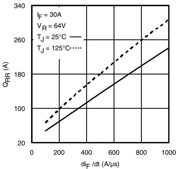
**Fig. 19** - Typical Stored Charge vs.  $di_f/dt$
