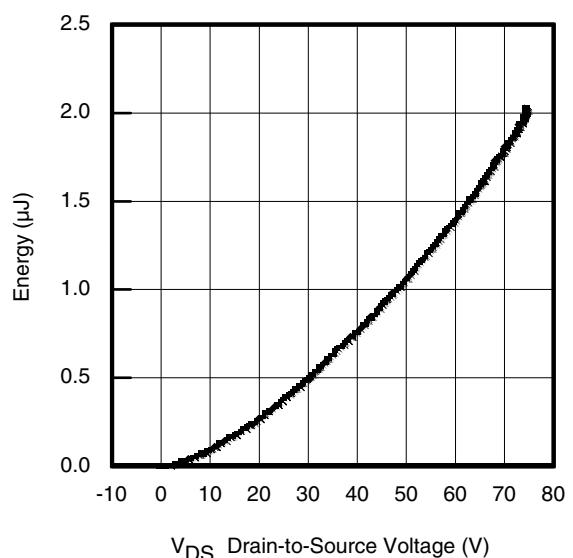
**Fig 11.** Typical  $C_{oss}$  Stored Energy
