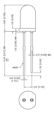
\*UNLESS OTHERWISE SPECIFIED TOLERANCES PER DECIMAL PRECISION ARE: X=±1 (±0.039), XX=±0.5 (±0.020), XXX=±0.25 (±0.010), XXXX=±0.127 (±0.005). LEAD SIZE=±0.05 (±0.002), LEAD LENGTH=±0.75 (±0.030). MIN=  $\frac{+0.00}{-0.00}$  MAX.=  $\frac{+0.00}{-0.00}$  MAX
