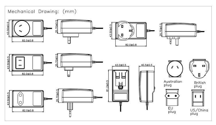
A full set of connectors is delivered with each product order. If a specific connector Is required then add a U,A,E or B to the I suffix on your order.
