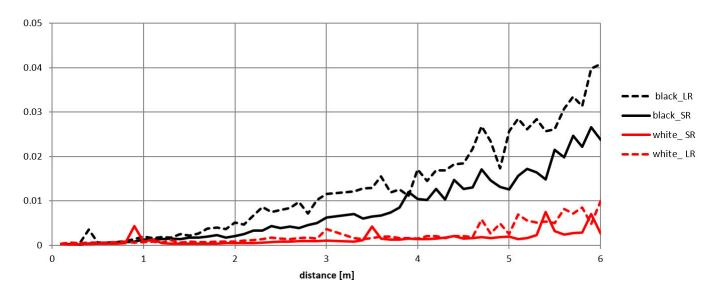
Sigma of binned distance [m] up to 6 m for short and long range mode
