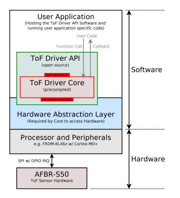
Figure 13 shows the software architecture overview for the basic implementation of the ToF Driver Core into user hardware and software. The precompiled core is embedded into open source API layers, providing an interface to the user application. A hardware interface declares the required hardware access for the ToF driver core to the underlying hardware and peripherals. The latter is required to connect the core to the AFBR-S50 ToF sensor hardware through the SPI and GPIO interfaces.
