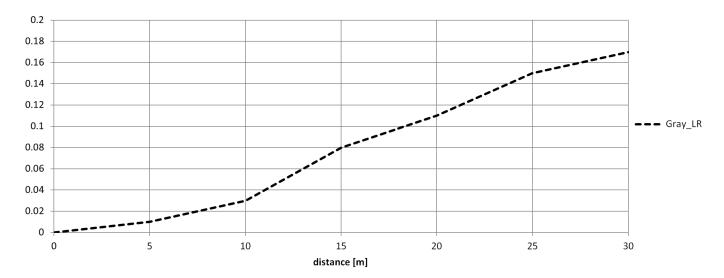
Sigma of binned distance [m] up to 30 m for long range mode
