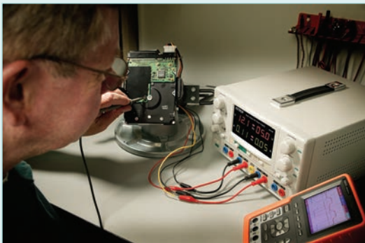
Single power supply with multiple DC outputs
