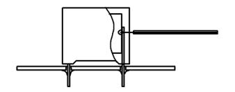
Temperature monitored inside the capacitor.
