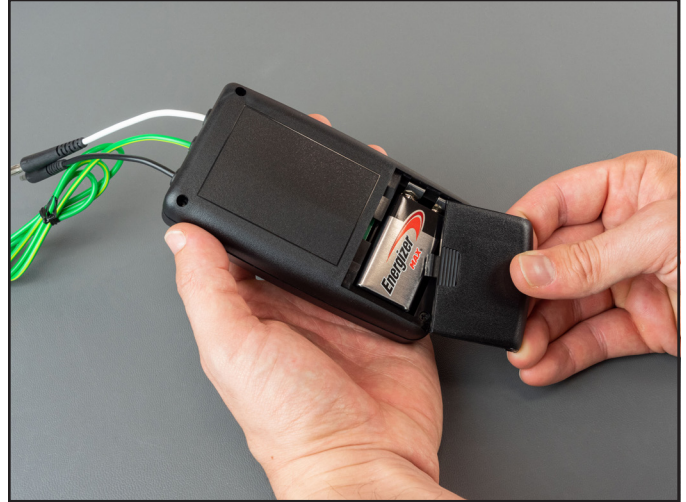
Figure 6. Removing the battery cover located on the back of the 724 Plus Monitor Verification Tester
