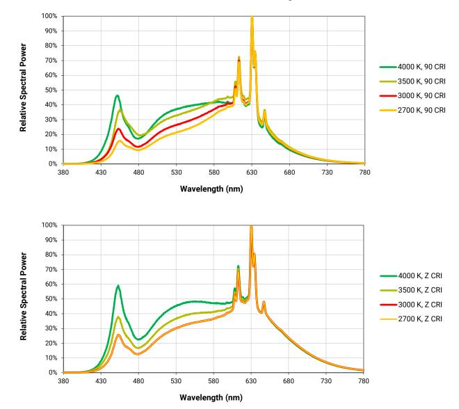
The following graphs are the result of a series of pulsed measurements at 270 mA and T<sub>1</sub> = 85 °C.
