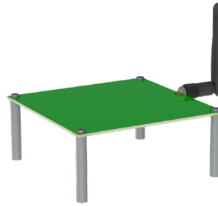
Bent 90°, on edge of ground
