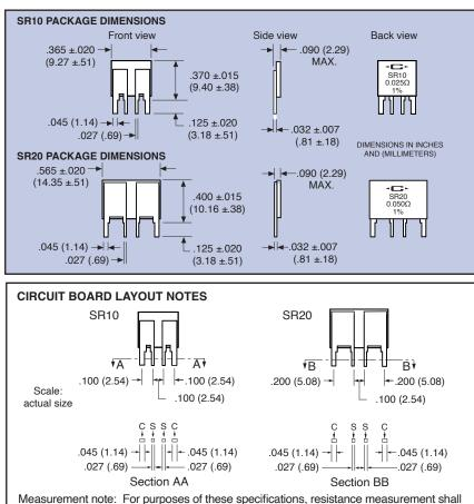
Measurement note: For purposes of these specifications, resistance measurement shall be made using Kelvin connections (four wire) with appropriate current and sense connections to the device terminals.
