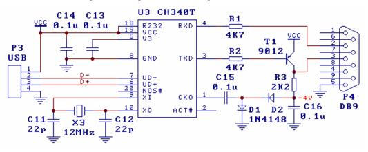
**7.3** USB to RS232 Converter Configuration (Simplified version using R232)
