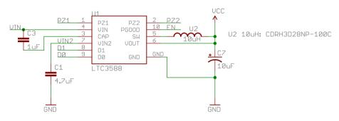
On the board 1 is VIN and 0 is GND 0 is default
