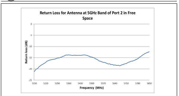
FIGURE 4.3.5 RETURN LOSS OF ANTENNA AT 5GHZ BAND OF PORT 2 IN FREE SPACE
