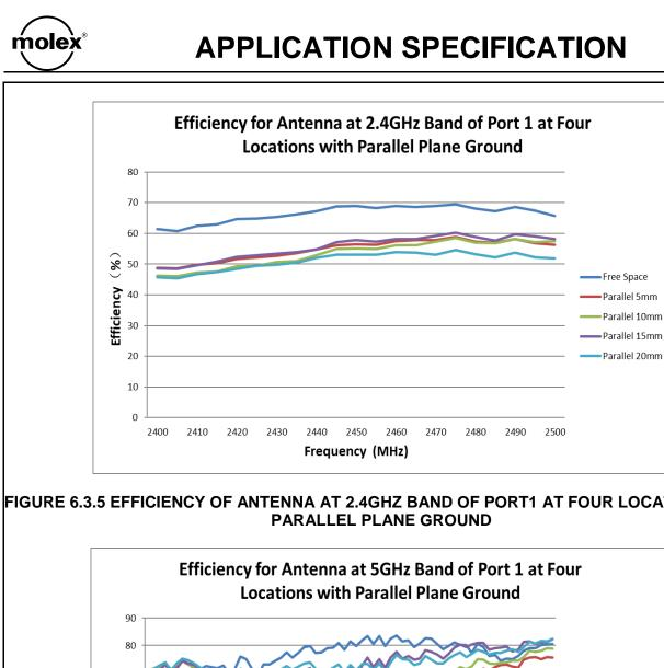
FIGURE 6.3.5 EFFICIENCY OF ANTENNA AT 2.4GHZ BAND OF PORT1 AT FOUR LOCATIONS WITH
