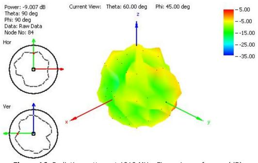
**Figure 16.** Radiation pattern at 1910 MHz, Figure 1 as reference (dB), with 2 m RG174 cable and free space
