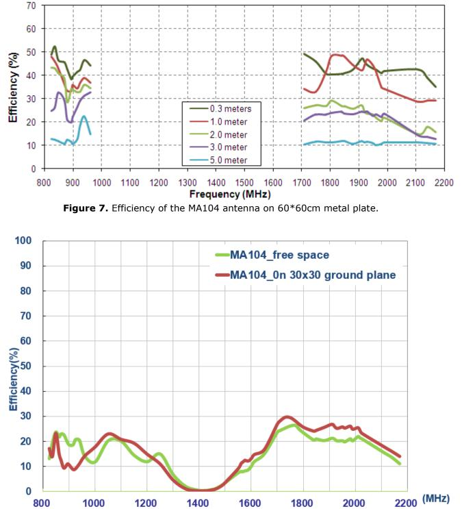
Figure 8. Efficiency of the MA104 antenna with 960~1700MHz
