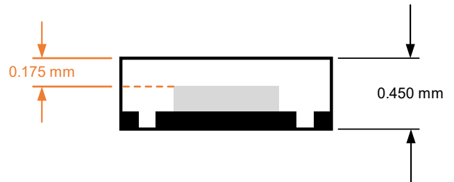
Figure 12. XtremeSense TMR Sensor Location in z Dimension for CT310 in DFN-8 Package
