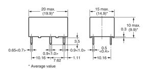
Dimensions in pointed brackets < > are for the Relay mounted to Socket(-P6C).
