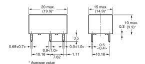
Dimensions in pointed brackets < > are for the Relay mounted to Socket(-P6C).
