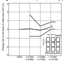
Sample: G6C-2114P-US DC24V Number of Relays: 6 pcs Test conditions: Shock is applied in ±X, ±Y, and ±Z directions three times each with without energizing the Relays to check the number of malfunctions.
