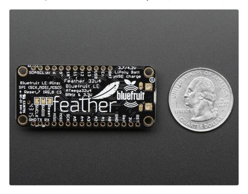
To make it easy to use for portable projects, we added a connector for any of our 3.7V Lithium polymer batteries and built in battery charging. You don't need a battery, it will run just fine straight from the micro
