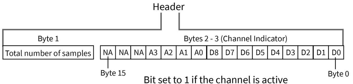
Sample data follows the header and the channel indicator frame determines how to read the sample data. If any of the DIO lines are enabled, the first two bytes are the DIO sample. The ADC data follows. ADC channel data is represented as an unsigned 10-bit value right-justified on a 16-bit boundary. The following figure illustrates the sample data bits.
