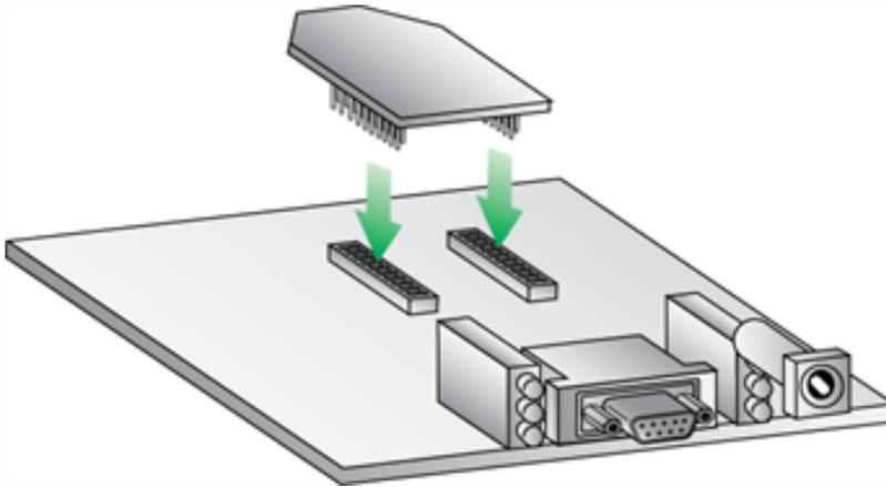
Century Interconnect and Samtec manufacture the 2 x 10 pin 2 mm spacing receptacles on Digi development boards. Several other manufacturers provide comparable mounting solutions; we currently use the following receptacles:
