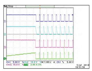
Output Short Circuit Protection V1
