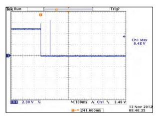
Output Short Circuit Protection V2
