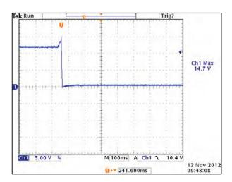
Output Short Circuit Protection V3
