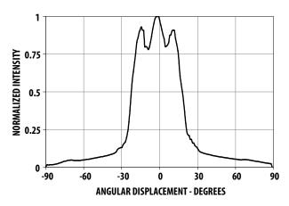
Figure 4. Relative Luminous Intensity vs. Angular Displacement for HLMP-Y651, HLMP-Y601, HLMP-Y951 and HLMP-Y701.
