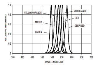
Figure 6. Wavelength vs. Relative Luminous Intensity.
