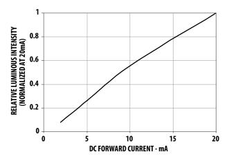
Figure 2. Relative Luminous Intensity vs. Forward Current.
