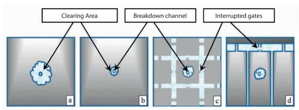
a and b: not segmented metallization; c and d: examples of segmented metallization. Effects of clearing on the two different film metallization designs.
