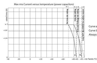
Curve a: DCB, DCH, DCS, PHC, RHB, RMC, PPS, PPA, RSB, RMB, MAR. Curve b: other series for power applications.
