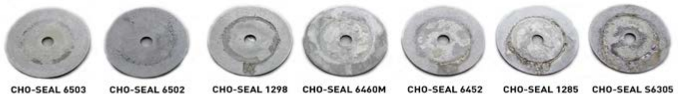
Figure 2-2 Picture of Corrosion Coupon After 504 hours salt spray / salt fog
