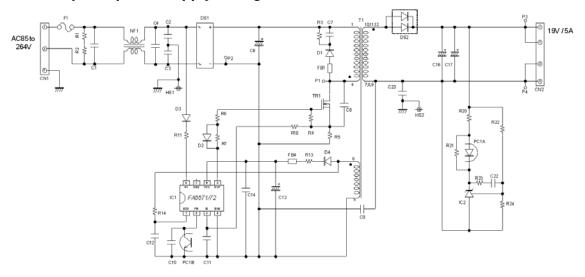
Standby power and efficiency (power supply specifications: output power - 19V, rating - 5 A)
