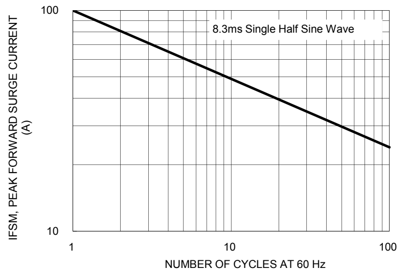
FIG. 4 MAXIMUM NON-REPETITIVE FORWARD SURGE CURRENT UNIDIRECTIONAL ONLY
