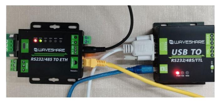
Open the <u>TCPIP/UDP debugging software</u>, set the computer as the server, RS232/485
