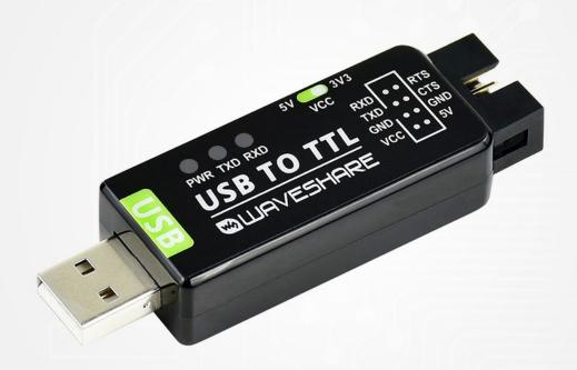
Industrial USB TO TTL Converter, Original FT232RL Onboard, Embedded Resettable Fuse, and ESD / IO Protection Diodes, Small Form Factor
