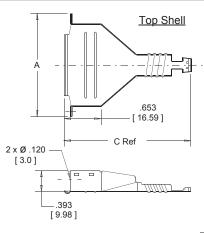
Inch [mm] Tolerance Unless Noted .000 Inch ±.01 ±.005 ±.1 [] Dimensions for Reference Only
