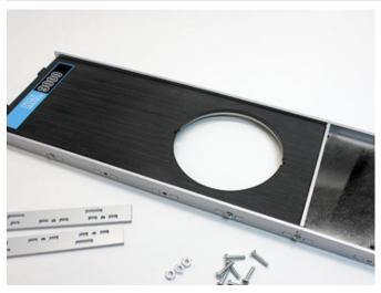
The front face then slots into place, and the top edge of the frame can be installed. Note that this piece only has tabs on the top and bottom, in order to minimize the number of holes along the frame (the button will be helping support it).
