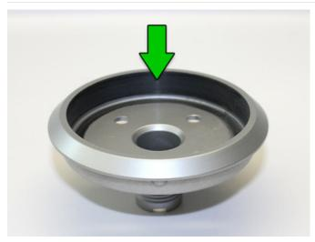
If you do decide on the black outer ring, you'll probably want the inside edge of the bezel to be free of paint, otherwise it rubs off when the button is pressed (as it inevitably will be). You can either sand this away (as shown here), washing and drying completely afterward, or with forethought could mask off this edge with tape before spray painting.
