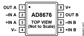
Figure 2. 8-Lead MSOP (RM-8)
