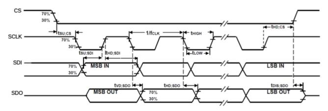
Figure 2 SPI Bus Timing Diagram
