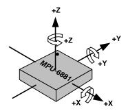
Figure 13 Orientation of Axes Sensitivity and Polarity of Rotation
