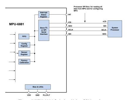
Figure 7 MPU-6881 Solution Using SPI Interface
