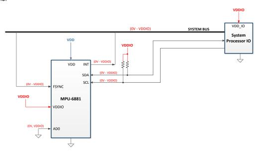
Figure 12 I/O Levels and Connections
