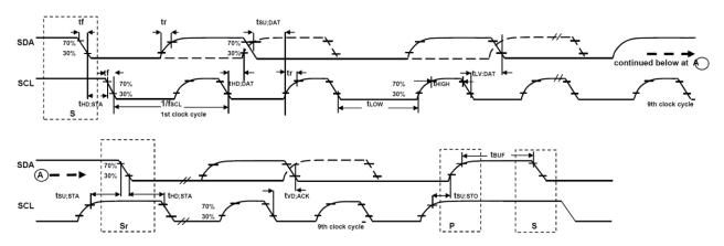
Figure 1 I2C Bus Timing Diagram
