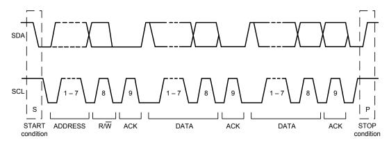
Figure 10 Complete I<sup>2</sup>C Data Transfer
