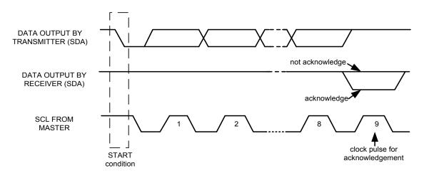
Figure 9 Acknowledge on the I<sup>2</sup>C Bus
