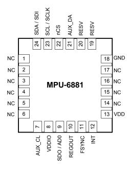
Figure 3 Pin out Diagram for MPU-6881 3.0x3.0x0.9mm QFN
