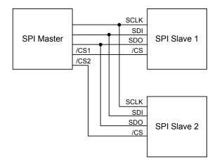
Figure 11 Typical SPI Master / Slave Configuration
