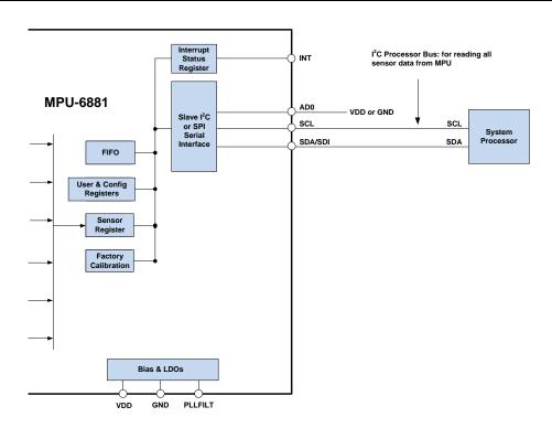
Figure 6 MPU-6881 Solution Using I2C Interface
