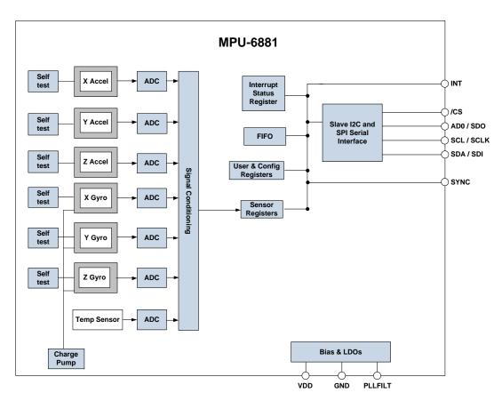
Figure 5 MPU-6881 Block Diagram
