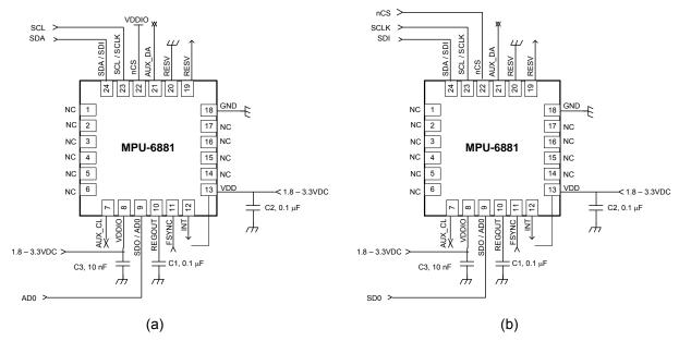
Figure 4 MPU-6881 QFN Application Schematic. (a) I2C operation, (b) SPI operation.
