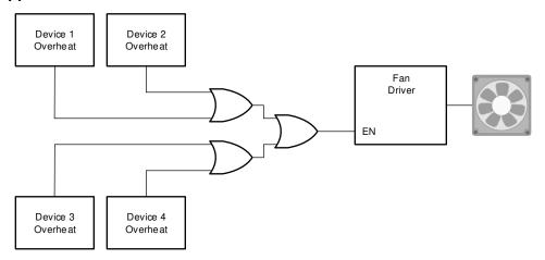
Figure 9-1. Typical application schematic
