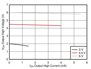
Figure 6-1. Typical output voltage in the high state  $(V_{OH})$
