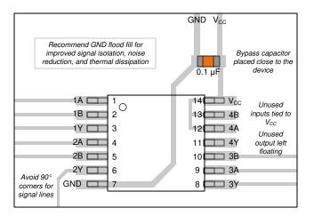
Figure 9-1. Example layout for the SN74HC32
