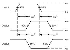
The maximum between  $t_{PLH}$  and  $t_{PHL}$  is used for  $t_{pd}$ . Α.
