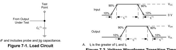
A. C<sub>L</sub>= 50 pF and includes probe and jig capacitance.
