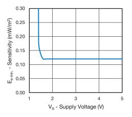
Fig. 13 - Sensitivity vs. Supply Voltage
