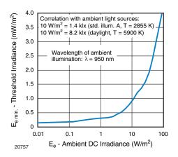
Fig. 6 - Sensitivity in Bright Ambient
