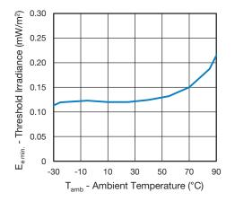
Fig. 9 - Sensitivity vs. Ambient Temperature
