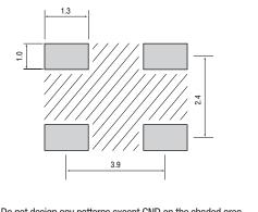
Do not design any patterns except GND on the shaded area. Except for this recommended soldering pattern, please contact us for inquiries.
