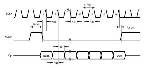
Figure 2. Serial Timing Diagram
