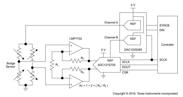
Figure 38. Driving an ADC Reference
