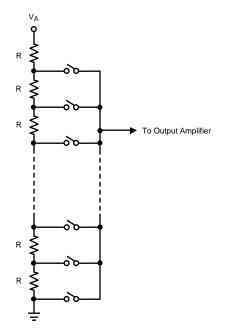
Figure 31. DAC Resistor String
