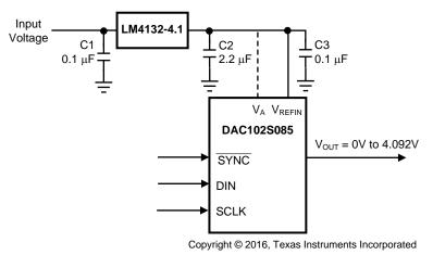
Figure 40. The LM4130 as a Power Supply
