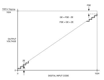
Figure 1. I/O Transfer Characteristic
