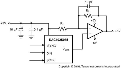
Figure 37. Bipolar Operation
