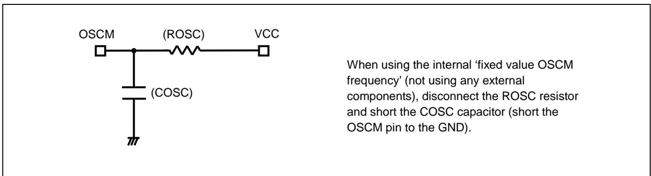
Note: The equivalent circuit diagrams may be simplified or omitted for explanatory purposes.
