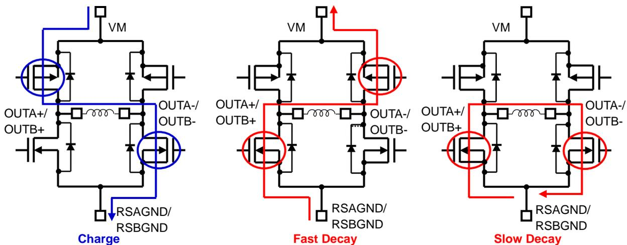
Note: Fixed value of 400 ns (design value) is prepared at the switching timing of MOSFET output to avoid any flow-through current. The equivalent circuit diagrams may be simplified or omitted for explanatory purposes.
