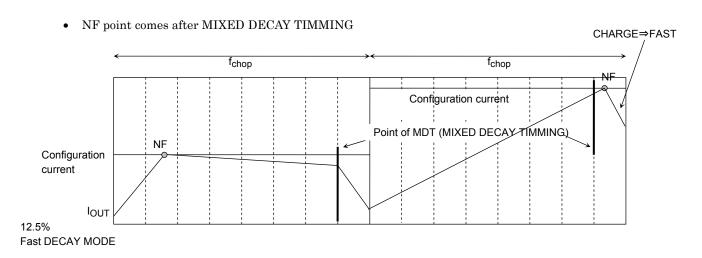
• MIXED DECAY MODE: Output current > Configuration current
