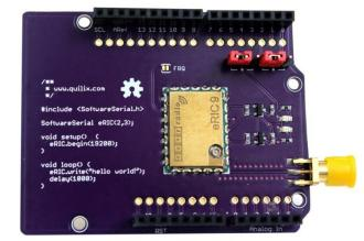
This 'shield' allows Arduino<sup>™</sup> boards to communicate wirelessly using proprietary LPRS 'easyRadio' technology operating in the 433MHz or 868/915MHz (Industrial Scientific & Medical (ISM) bands.
